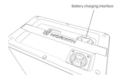
First connect the charger to the battery interface, and then to the socket. If the charging process does not start automatically, press the charging indicator button.
